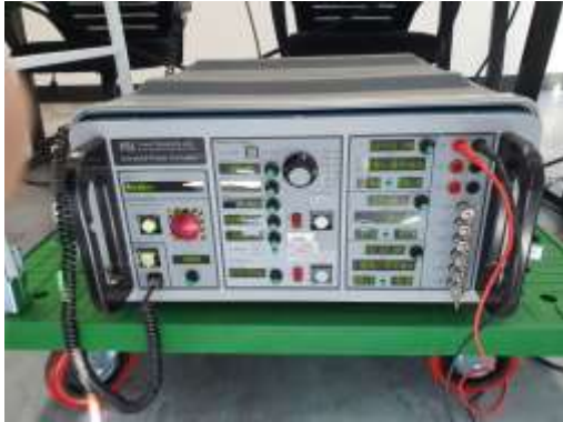
Photo 2: IPC Voltage Sag Generator
