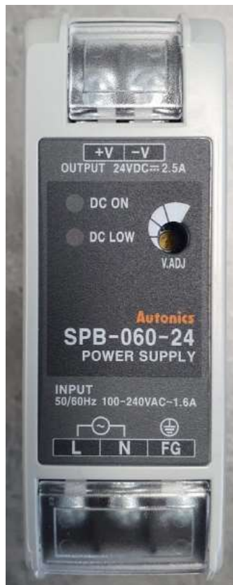
Photo 1: Equipment under test POWER SUPPLY / SPB-060-24
