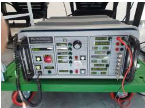
Photo 2: IPC Voltage Sag Generator
